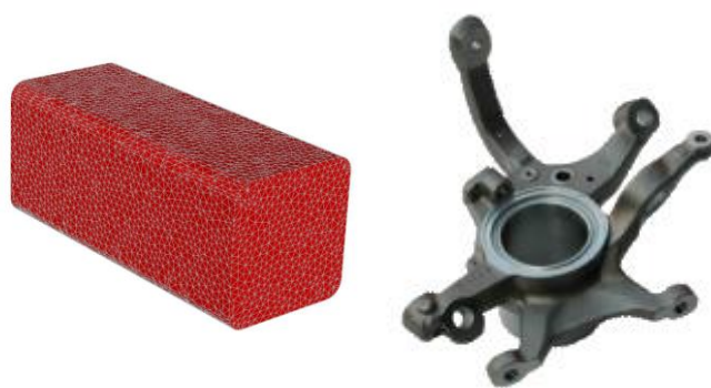
Figure 2: Input and output of the forging process
